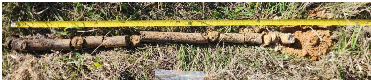
Figure 2-8: Typical soil profile across site: loamy-sand over sandy-silty-clay overlying granite
